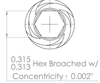
18.43° Lead Angle Right Hand Thread 25° Pressure Angle 4 Lead
